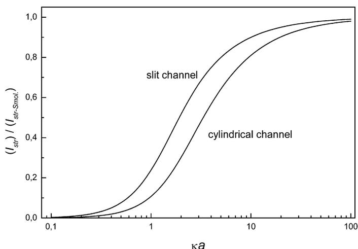
**Fig. 3** Streaming current divided by the applied pressure difference, eqs. 37 and 39, relative to the Smoluchowski formula, eq. 33, plotted as a function of the product  $\kappa a$  ( $a$ : capillary radius, or slit half-width) for slit- and cylindrical-shaped capillaries.
