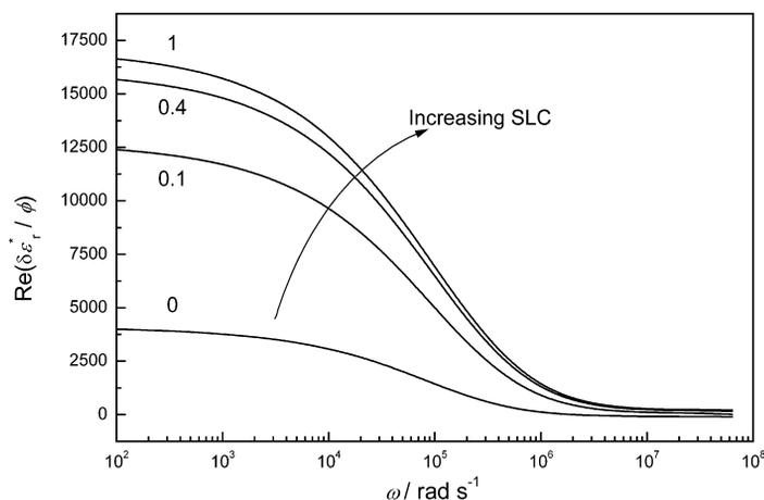
**Fig. 7** Real part of the dielectric increment (per volume fraction) of dilute suspensions as in Fig. 5. The curves correspond to increasing importance of SLC; the ratios between the diffusion coefficients of counterions in the stagnant layer and in the bulk electrolyte are indicated (the lower curve corresponds to zero SLC).
