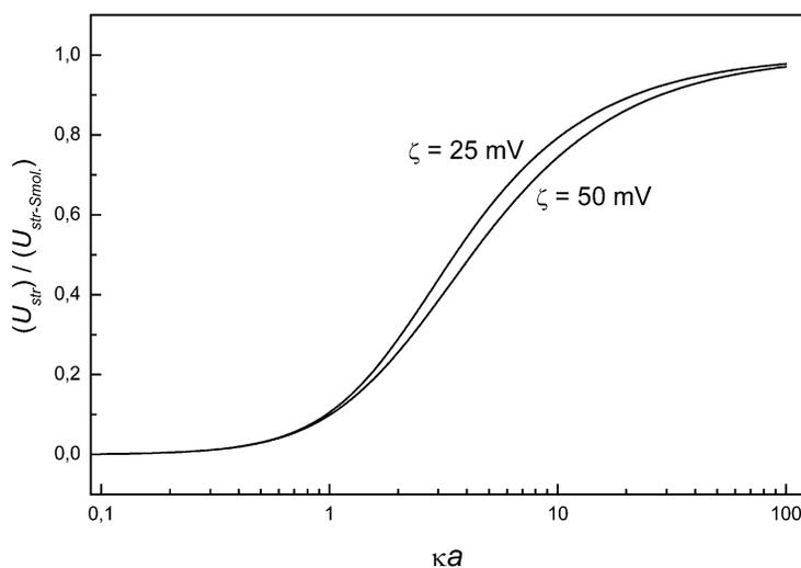
**Fig. 4** Streaming potential divided by the applied pressure difference, eq. 44, relative to its Smoluchowski value, eq. 40, as a function of the product  $\kappa a$  ( $a$ : capillary radius), for the  $\zeta$ -potentials indicated. Surface conductance is neglected.
