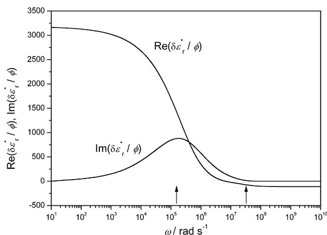
**Fig. 5** Real and imaginary parts of the dielectric increment  $\delta\epsilon_r^*$  (divided by the volume fraction  $\phi$ ) for dilute suspensions of 100-nm particles in KCl solution, as a function of the frequency of the applied field for  $\kappa a = 10$  and  $\zeta = 100$  mV. The arrows indicate the approximate location of the  $\alpha$  (low frequency) and Maxwell–Wagner–O’Konski relaxations.
