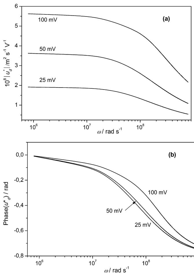
**Fig. 8** Modulus (a) and phase angle (b) of the dynamic mobility of spherical particles in a KCl solution with  $\kappa a = 20$  as a function of frequency for different  $\zeta$ -potentials; cf., eqs. 80–82. Parameters: particle radius 100 nm; dielectric constant of the particles (dispersion medium): 2 (78.54); density of the particles (dispersion medium):  $5 \times 10^3$  ( $1 \times 10^3$ )  $\text{kg m}^{-3}$ .
