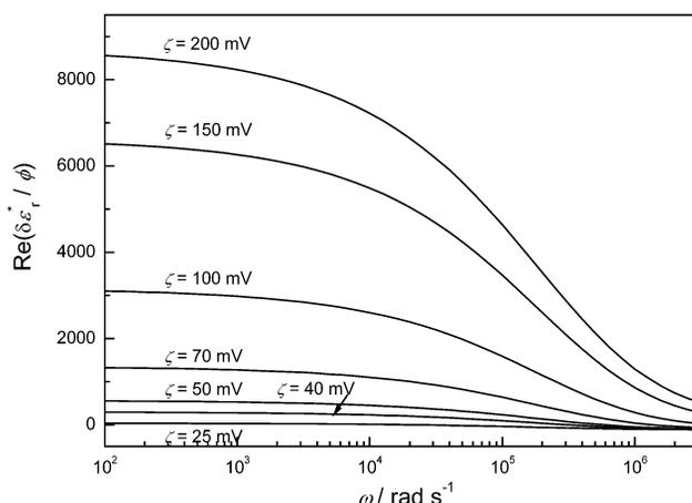
**Fig. 6** Real part of the dielectric increment  $\delta\epsilon_r^*$  (per volume fraction) as a function of the frequency of the applied field for dilute suspensions of 100-nm particles in KCl solution. The  $\zeta$ -potentials are indicated, and in all cases,  $\kappa a = 10$ .
