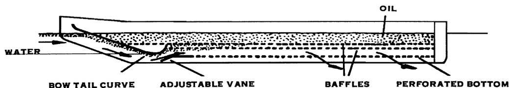
Fig. 4 Combination oil skimmer/separator.
