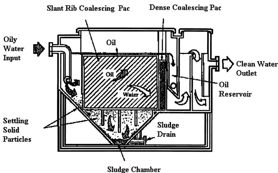
Fig. 2 Slant rib coalescing separator.
