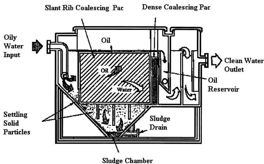
Fig. 2 Slant rib coalescing separator.
