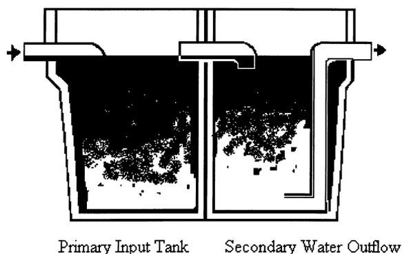
Fig. 1 Basic type gravity separator.
