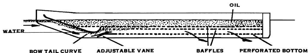
Fig. 4 Combination oil skimmer/separator.
