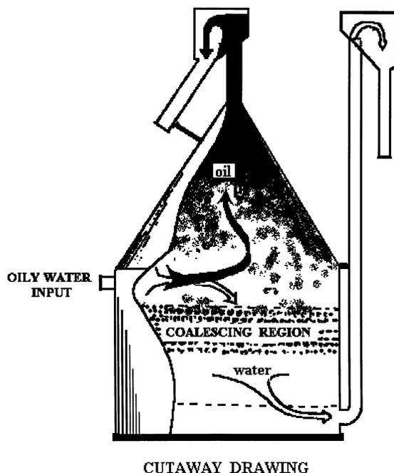
Fig. 3 Inverted cone separator.
