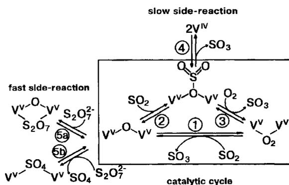
Scheme 2. The mechanism of  $\text{SO}_2$  oxidation to  $\text{SO}_3$  over industrial vanadium catalysts.
