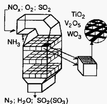
Fig. 6. Reactor and honeycomb catalyst for the catalytic reduction of NO<sub>x</sub> in flue gases of power plants.
