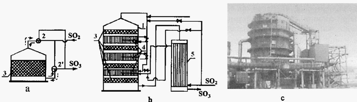
Fig. 7. Schemes and relative sizes of catalytic reactor and heat exchanger units for unsteady-state (a) and traditional steady-state (b) performance of  $\text{SO}_2$  removal from flue gases of non-ferrous metal plants (1 - reactor, 2 and 2' - three way valves; 3 - catalyst beds; 4 and 5 - heat exchangers). Photograph of the industrial unit for unsteady-state  $\text{SO}_2$  removal (c).
