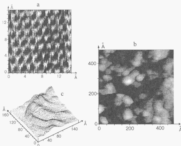
**Fig. 1.** STM images of: (a) - the basal surface of graphite; (b) - the surface of Pd/Sibunit catalyst with highly dispersed Pd particles; (c) - the surface of a large Pd particle in Pd/Sibunit catalyst.
