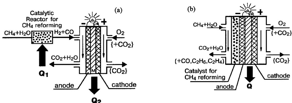
**Fig. 4.** High output methane fuel cells with the external (a) and internal (b) reforming of CH<sub>4</sub>. Thick arrows indicate heat fluxes. M is the high-temperature oxygen conducting membrane or molten carbonate.
