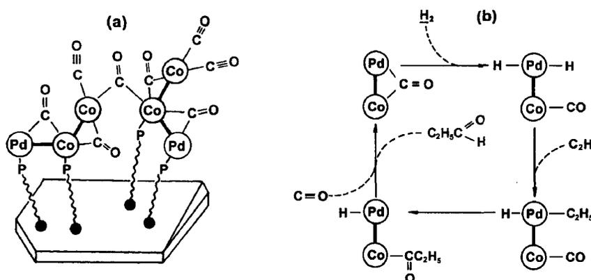
Fig. 2. Active site of the bimetallic (Pd+Co)/SiO<sub>2</sub> catalyst (a) and the mechanism of hydroformylation of ethylene over this site (b)
