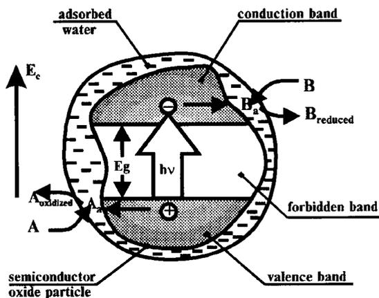
Fig. 9. Photogeneration of the holes and electrons at the aerosol semiconductor particle under light with  $h\nu > E_g$  and subsequent redox processes that provide the overall reaction:  $A + B \longrightarrow A_{\text{oxidized}} + B_{\text{reduced}}$ .
