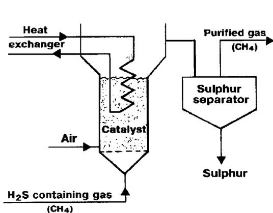
Fig. 8. Reactor with fluidized catalyst bed for selective oxidation of hydrogen sulfide.
