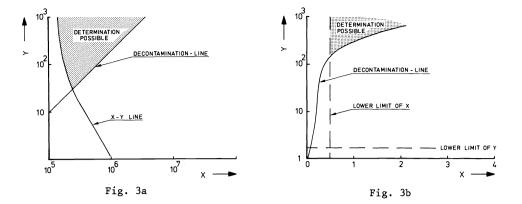
Fig.3a. The X-Y graph for the determination of mercury in air.
