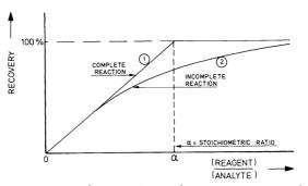
Fig.1. The recovery as a function of the ratio mass of reagent/mass of analyte.
